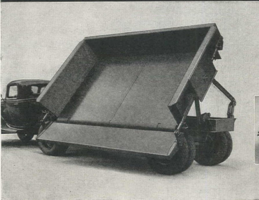
Hydraulic controls from the cab dump the body to (either side) while drop doors act as a chute to clear the load.
