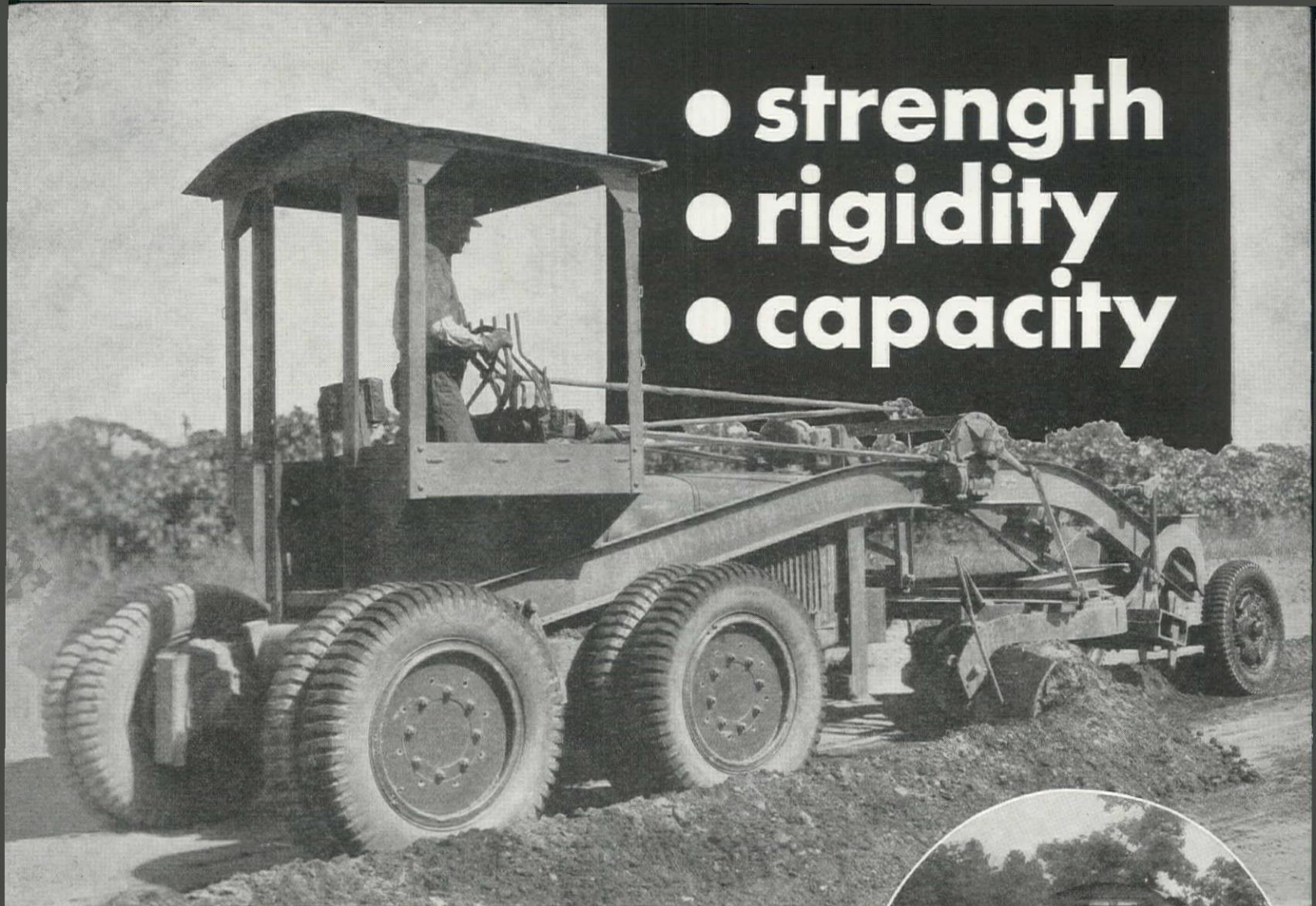
Adams Motor Grader—8-wheel Tandem Drive—mixing oil and sand.
