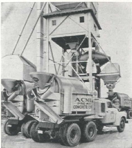
A WINNING COMBINATION — Smith Tiltting Mixers for pre-mixing or pre-shrinking concrete and Smith-Mobile Agitators for delivering the concrete to the job.
