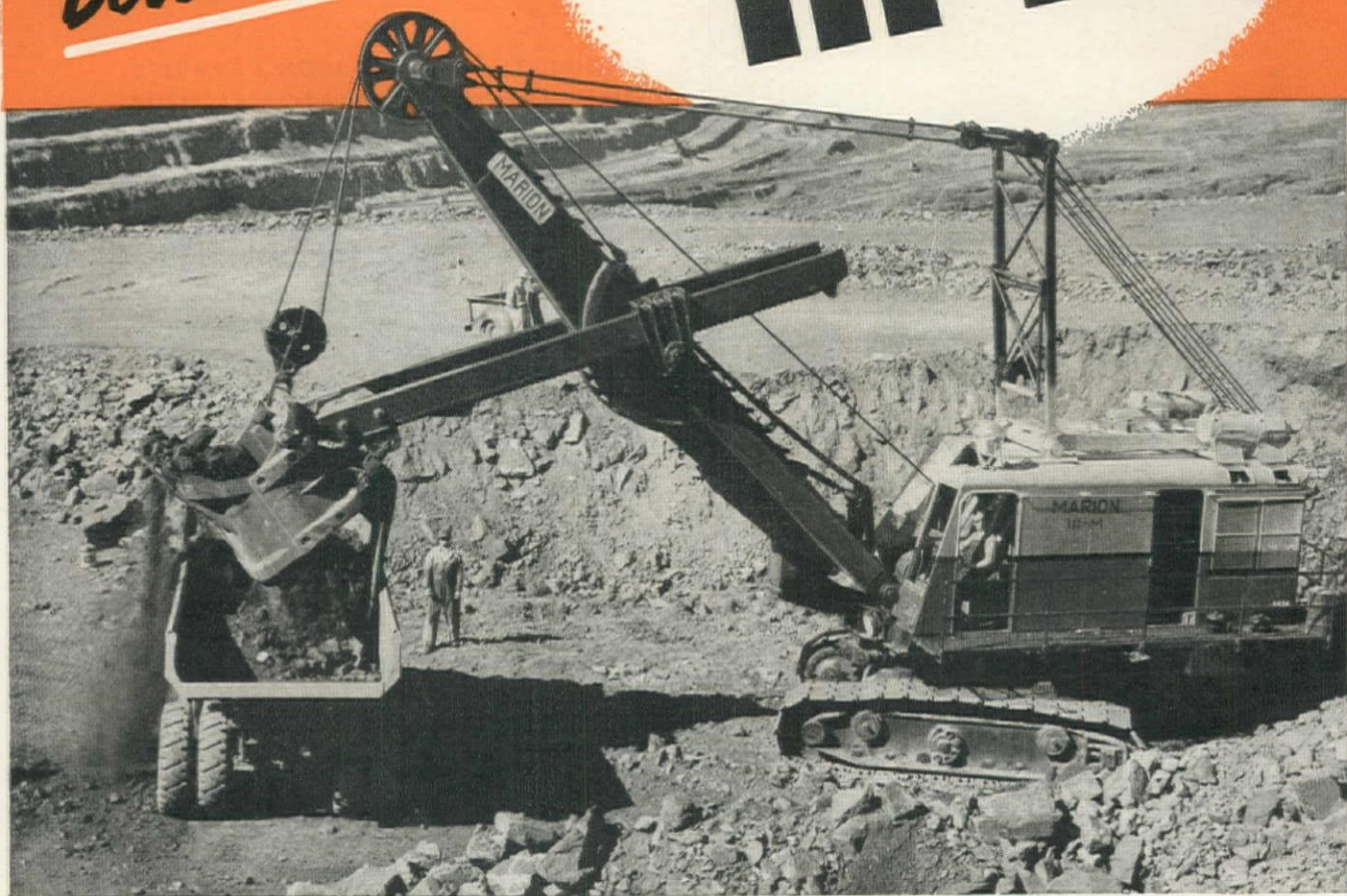
Machine illustrated has Diesel power with electric swing. Also available as full Ward-Leonard Electric machine.
