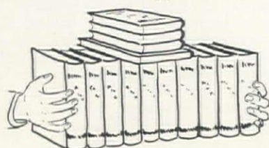
A simple analogy—squeezed together, a "beam" of books can support a load.
