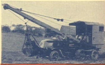
Motor Truck (Christie) Crawler com- bines crawler traction and motor truck speed with reduction of wheel loads.
