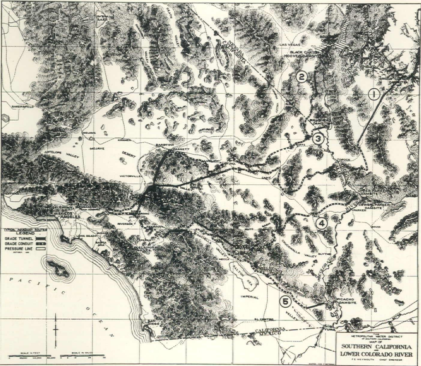
FIG. 4. FOUR ALTERNATE ROUTES FOR COLORADO RIVER AQUEDUCT RECOMMENDED BY ENGINEERING BOARD FOR CONCENTRATED STUDIES
