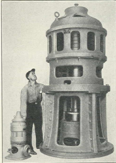
Driving Head and Westinghouse Motor for Pomona Deep Well Turbine Pump, 850-ft. Lift
