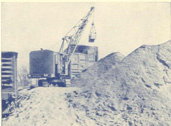
P & H Model 300-A equipped with clamshell bucket handling sand for Commerce Street viaduct.
