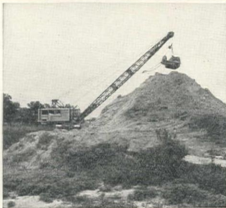
The stability and power of the machine make it easy to handle a 60-ft. boom and 2-yard bucket.
