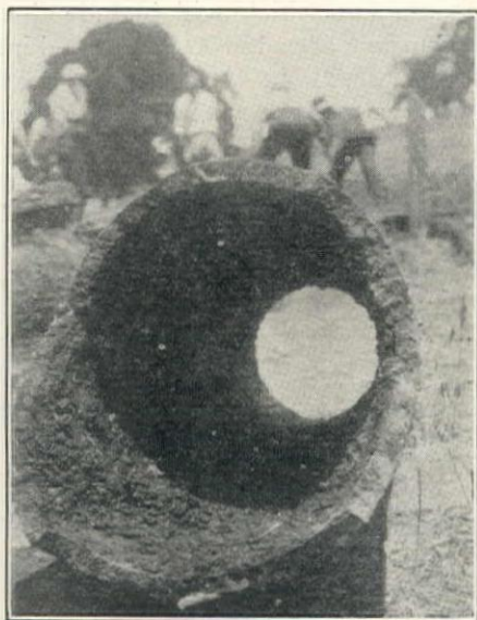
Fig. 1. Tubercles on Section of 12-in. Cast-Iron Irrigation Supply Line for Stanford University. Pipe in Service 38 Years Before Cleaning
