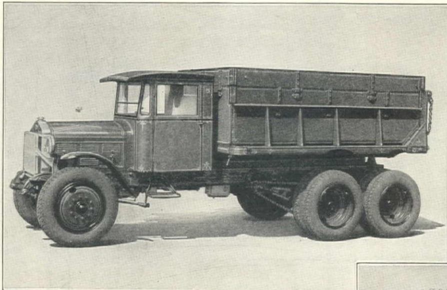
For grueling, heavy work . . . STERLING DC-26 . . . a heavy duty, six cylinder chain drive unit.
