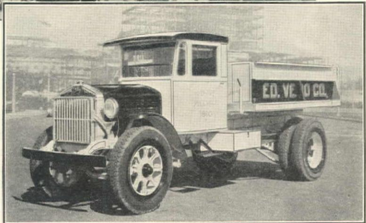
Tremendous pulling power, for heavy hauling at a profitable speed... Sterling DC-23, 5½ to 7 ton, chain drive.
