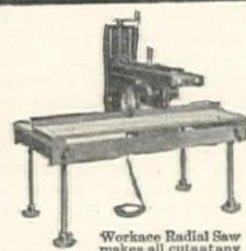
Wallace Radial Saw makes all cuts at any angle. Saw travels through work.
