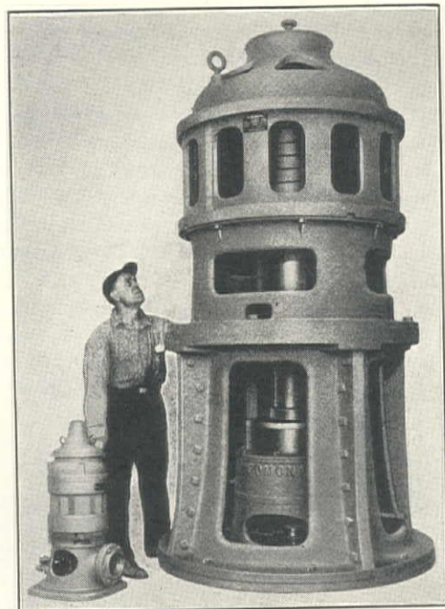
Driving Head and Westinghouse Motor for Pomona Deep Well Turbine Pump, 850-ft. Lift
