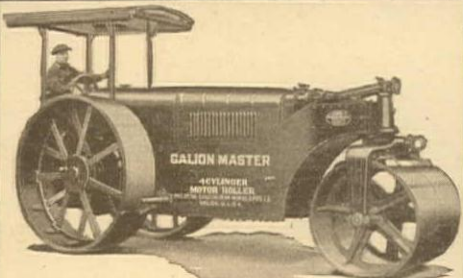
GALION MASTER 4-CYLINDER MOTOR ROLLER. 10 OR 12 TON
