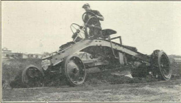
United Center-Control Grader, a 1-man Unit for Grading and Maintenance, Built by Wehr Co. and Powered with United Tractor
