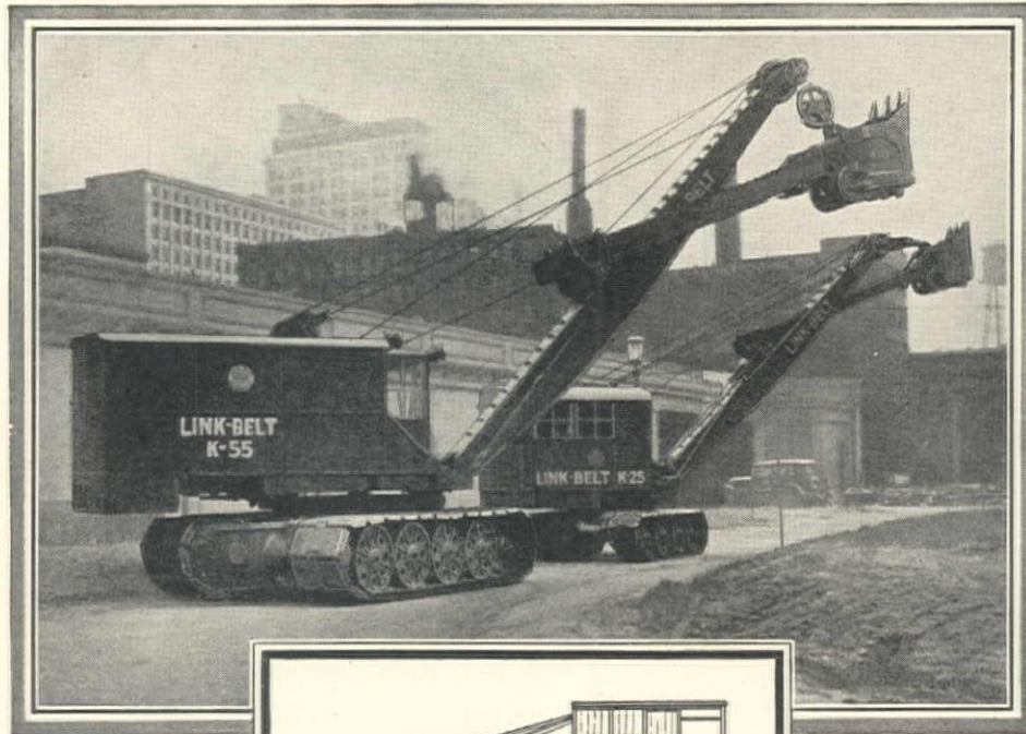
K-55, can be shipped loaded on a flat car without dismantling.
