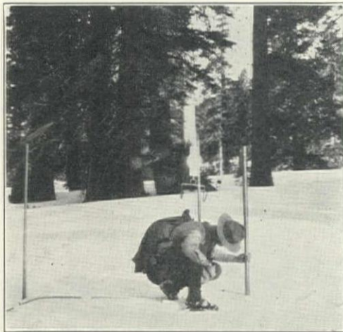
Observing Snow Depth by Means of Sample Tube
