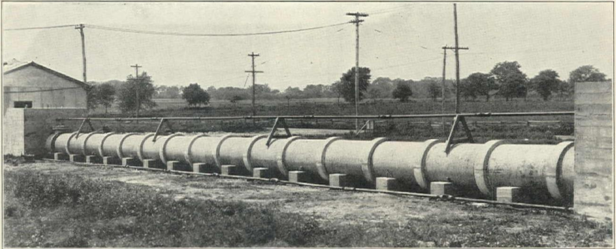
Demonstration Line Tested to 400 lb. Hydraulic Pressure without Leakage. This Pipe was Spun by the Moir-Buchanan Centrifugal Process, and Asphalt Lined by the Billé-Lignonnet Method.
