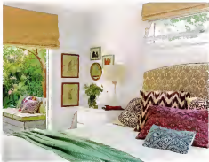
LEFT: Above the bed a large sliding window with a screen outside replaced two original windows that looked onto a neighbor's house. On the back wall, a pair of French doors now open onto a new deck, offering unobstructed views of the back garden as well as good cross ventilation when open at the same time as the window.
