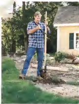
Roger Cook presents digging postholes with a Bosch digger, which can cut through solid holes nearly 4 feet deep.
