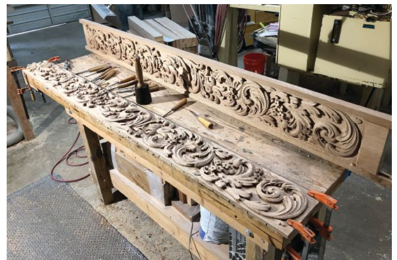
Top right, the overmantel had many broken and missing elements and had been modified to fit a much shorter room.
