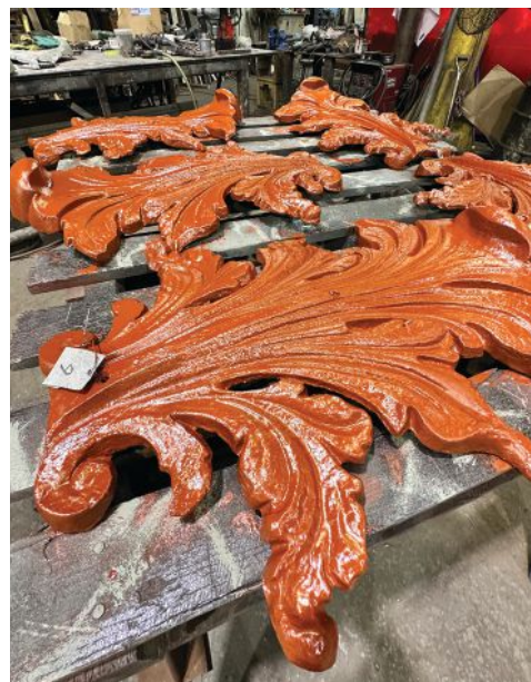
Robinson Iron disassembled the Court Square fountain for rehab in Alexander City. Fresh prime protects ornate cast iron in the shop. Above: Parts like basin got minor repairs before final finishes.
