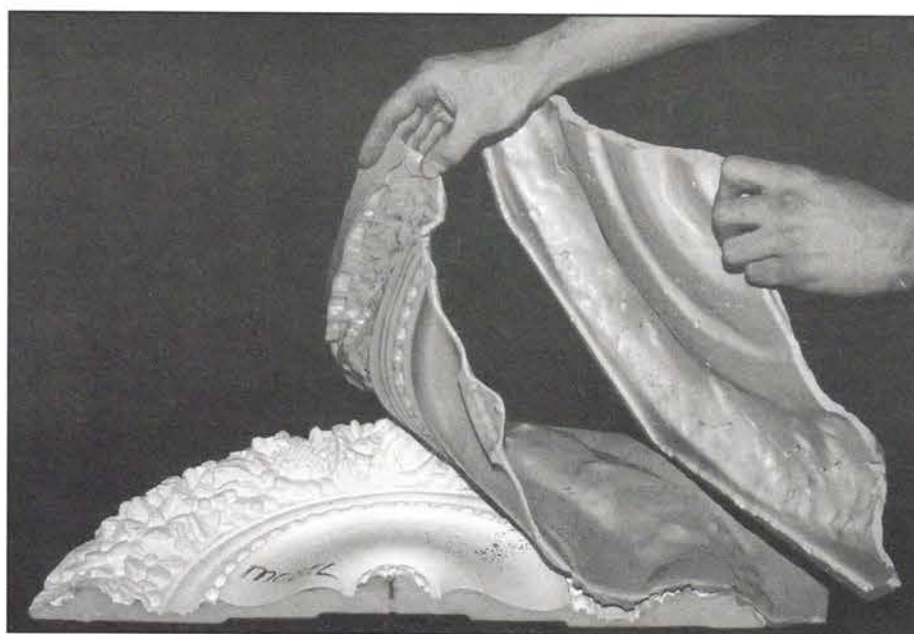
Polygel mold and Poly Resin shell by POLYTEK are shown here being used to create a production mold from the original model. Write in No. 636
