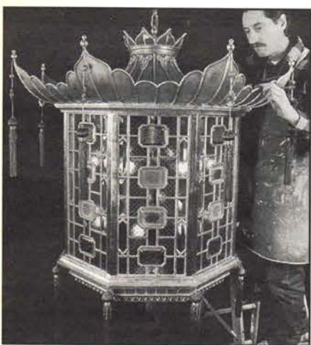
This light fixture is part of a series of Chinese lanterns molded in GRG for the Trump Taj Mahal project. The parts were assembled over a steel frame and finished with gold leaf and red crackle lacquer. Technology and polymer systems supplied by BALL CONSULTING. Write in No. 726
