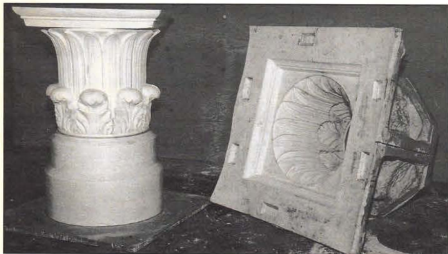
Column capital produced at PJR Industries, Kearney, NJ, using SMOOTH-ON's Brush-On 50 rubber mold compound for the production mold. Write in No. 65
