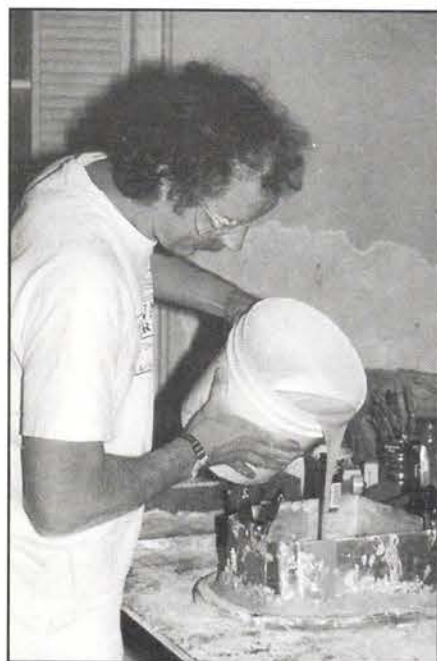
RORY BRENNAN is a specialist in restoring plaster ornament using traditional materials and methods. Above, Rory is pouring rubber for a mold to duplicate a plaster original. Write in No. 298
