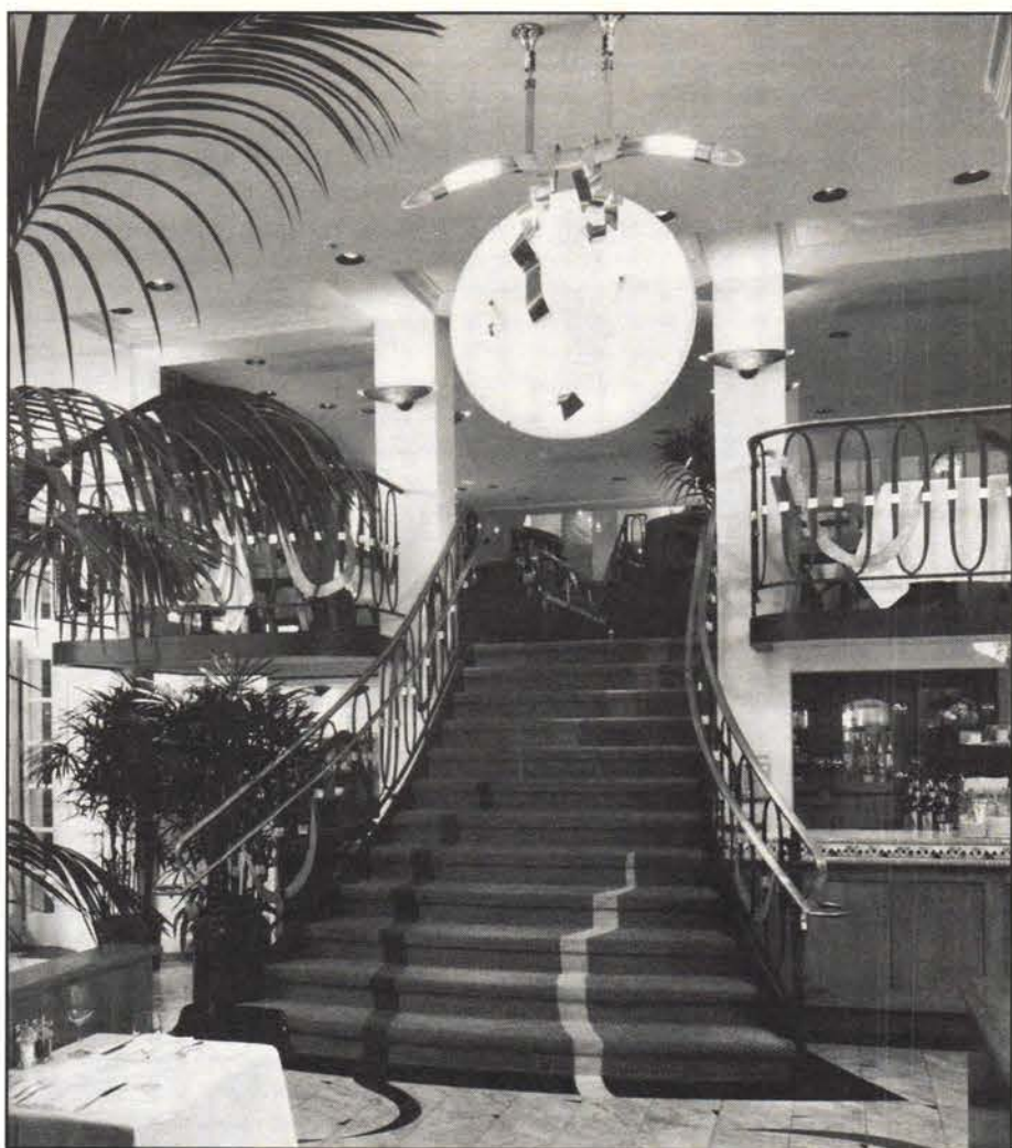
BONDI METAL DESIGN created this forged steel and copper stair rail with forged copper cap rail for the Wolfgang Puck Postrio Restaurant in San Francisco. Write in No. 752
