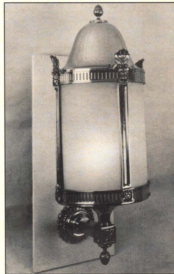
Fixture #1019. 12-in. dia. x 37-in. tall exterior wall sconce has a cast-brass body and decoration with large brass spinings top and bottom. Frosted acrylic tubing was used in place of glass to minimize cost of replacement in the event of vandalism.
