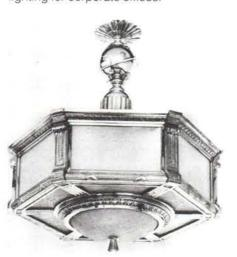
Lighting fixture made by The Steinmetz Co. to hang in a lower level hall of the U.S. Capitol. Made of cast brass, spun brass, and fluted brass tubing, it features etched glass on all 6 sides and bottom. It is 22" high to the column top, 19" across. Center of the bottom is hinged for bulb changing.
