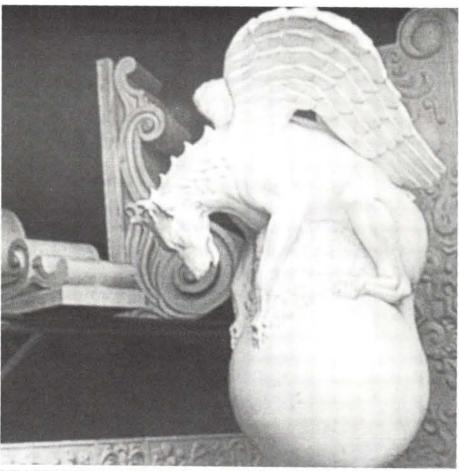
MJM STUDIOS created this fabulous gargoyle from an original design. Using SMOOTH-ON rubber mold compounds, a pair of them were cast in GFRC and now stand guard above an entrance to a building at 70th and Broadway in New York City. Write in No. 635 for MJM STUDIOS; No. 65 for SMOOTH-ON.
