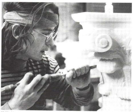
Skilled handcarvers at CATHEDRAL STONEWORKS provide the finishing touches on ornamental stone elements roughed in by a sophisticated CAD/CAM design and stone cutting system. Write in No. 935
