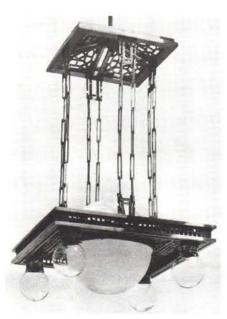
Frank Lloyd Wright designed this cast iron fixture for his 1905 renovation of The Rookery Building in Chicago. Ball & Ball was asked to renovate the 10 original units — and supply 6 new ones to match. The pattern in the fixture matches the rest of the iron lace in the building. A 19" square cast iron, brass-plated canopy trails 8 cast brass chains, 6 ft. long, supporting a 30" square main body, which in turn holds 4 corner globes and a central globe over and under the main body.
