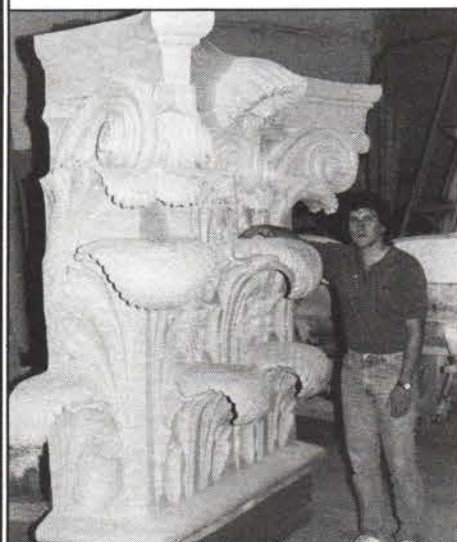
"After casting 10 large fiber-glass parts, the mold was in such good condition we could have made 50 more." The 8 ft. by 7 ft. corinthian column capitals have 24 inch undercuts.
