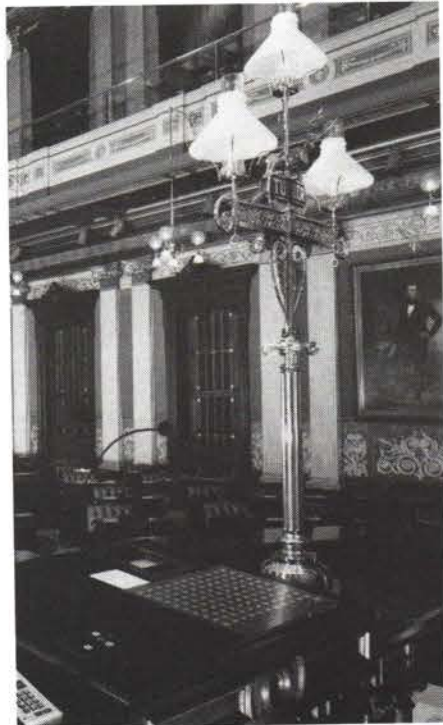
Light standards for the Michigan State Capitol were custom-cast in bronze via the lost-wax process by CIRECAST. Write in No. 593
