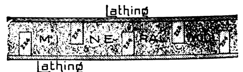
Section of sound-proof and fire-proof partition
