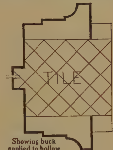
Showing buck applied to hollow tile partition
