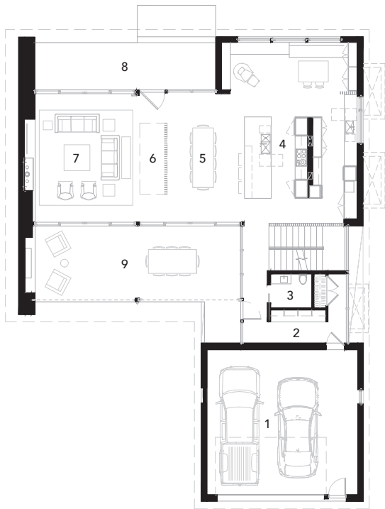
MAIN LEVEL PLAN | 1. Garage | 2. Mud | 3. Powder | 4. Kitchen | 5. Dining | 6. Entry | 7. Living | 8. Front Porch | 9. Patio
