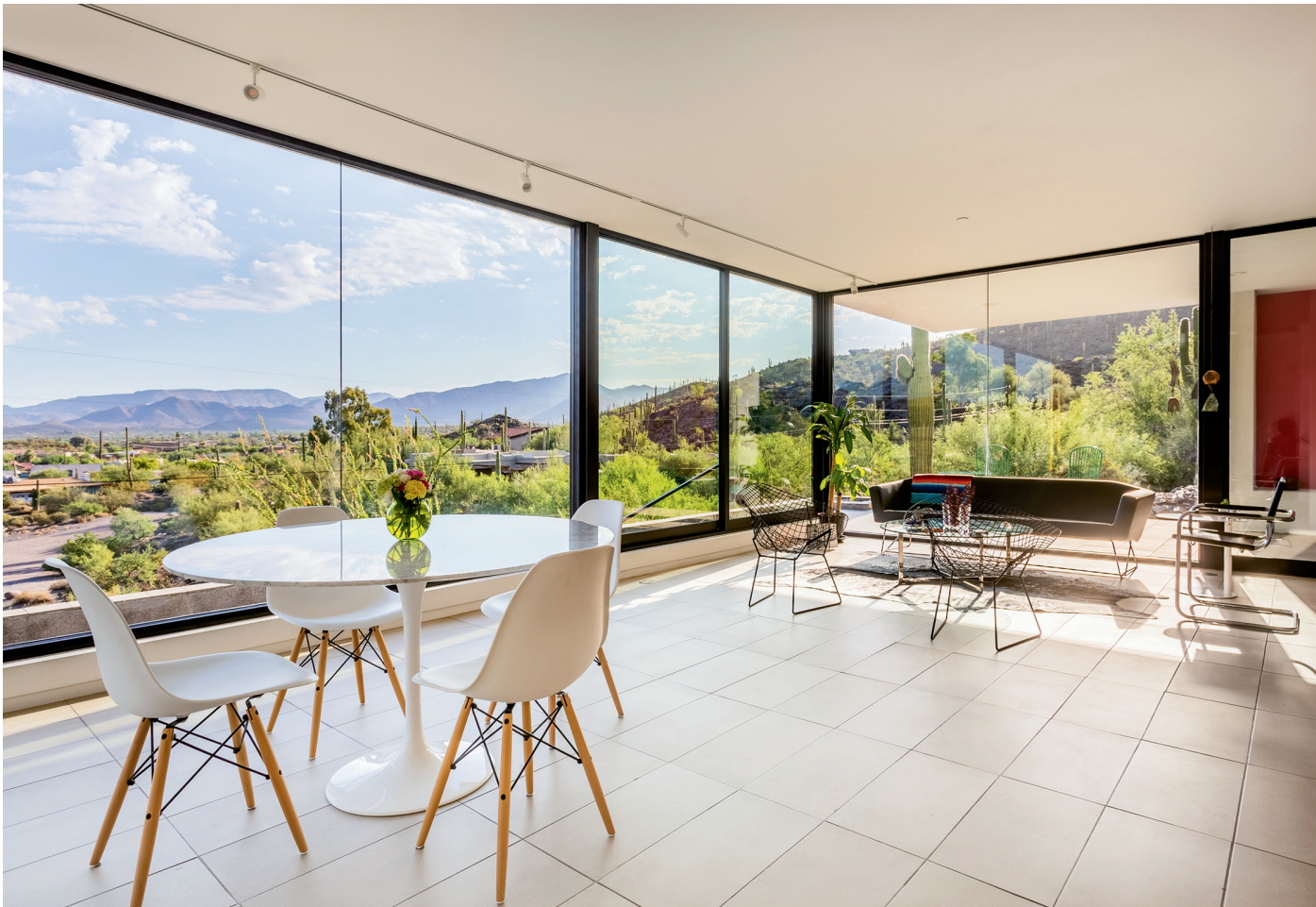
This page: Standard 8-foot-tall windows and sliders rest on the 8-inch-tall supporting beam for the house, achieving the minimum ceiling height needed for the interiors without the expense of custom units. Glazing is restricted to the north and east sides of the house to minimize heat gain. The durable gray floor tiles used throughout were just $3 a square foot.
