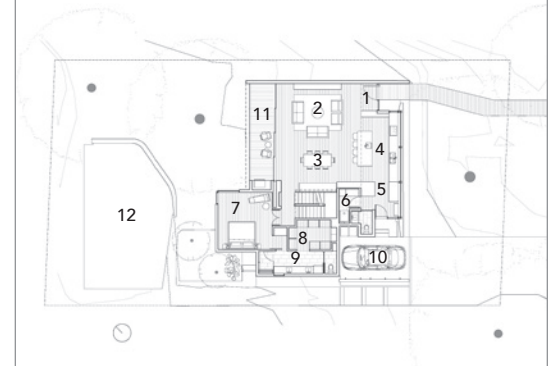
FIRST FLOOR PLAN | 1. Entry | 2. Living | 3. Dining | 4. Kitchen | 5. Mud | 6. Utility | 7. Primary Bedroom | 8. Primary Closet | 9. Primary Bath | 10. Carport | 11. Porch | 12. ADU Unit
