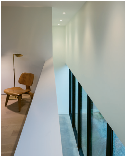
Light filters through the house and into the stairhall, second-level guest lounge, and bedrooms. A combination of fixed skylights and venting units control the flow of light and air. Behind the scenes, south walls are radiantly cooled to prevent excessive heat gain.
