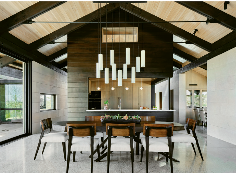
This page: The resort community required a minimum roof pitch, which the firm deployed like an abstracted tent form. Overhangs provide welcome shading for expansive walls of glass, while open gables convey light through the spaces. Rebecca designed the hand-carved alabaster light fixture over the dining table. High on the kitchen wall, a window draws light into a loft sitting area.
