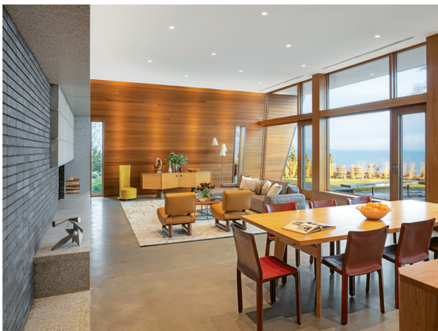
This page: Commonplace materials temper the scale of the large home. The fireplace combines dark, utility-grade Nelson bricks with lighter-colored concrete units and elevated granite hearth.
