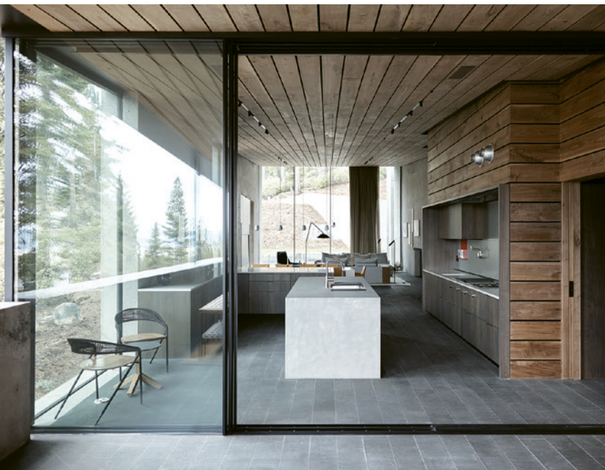
This page: 16-foot-tall, black steel window systems on the main-floor gather room are glazed in structural glass, allowing wide-open connections to covered and uncovered terraces. Indoor flooring segues outdoors, uniting both realms as continuous space.
