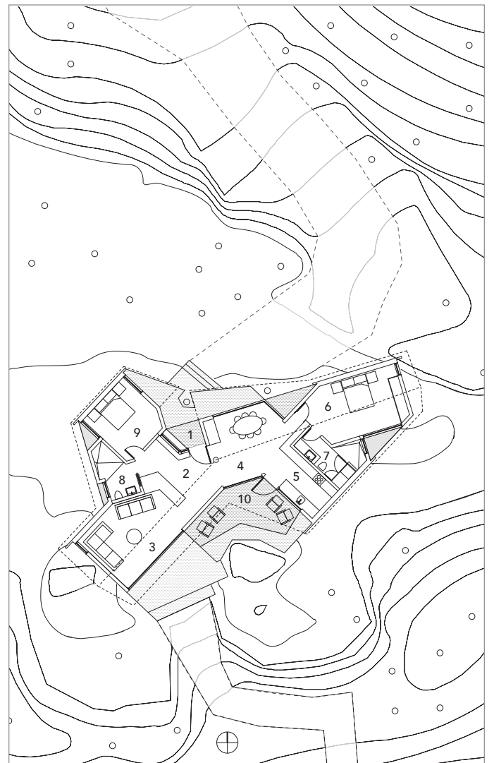
FLOOR PLAN | 1. Porch | 2. Entry | 3. Living | 4. Dining | 5. Kitchen 6. Main Bedroom | 7. En Suite | 8. Bathroom | 9. Guest Bedroom 10. Patio
