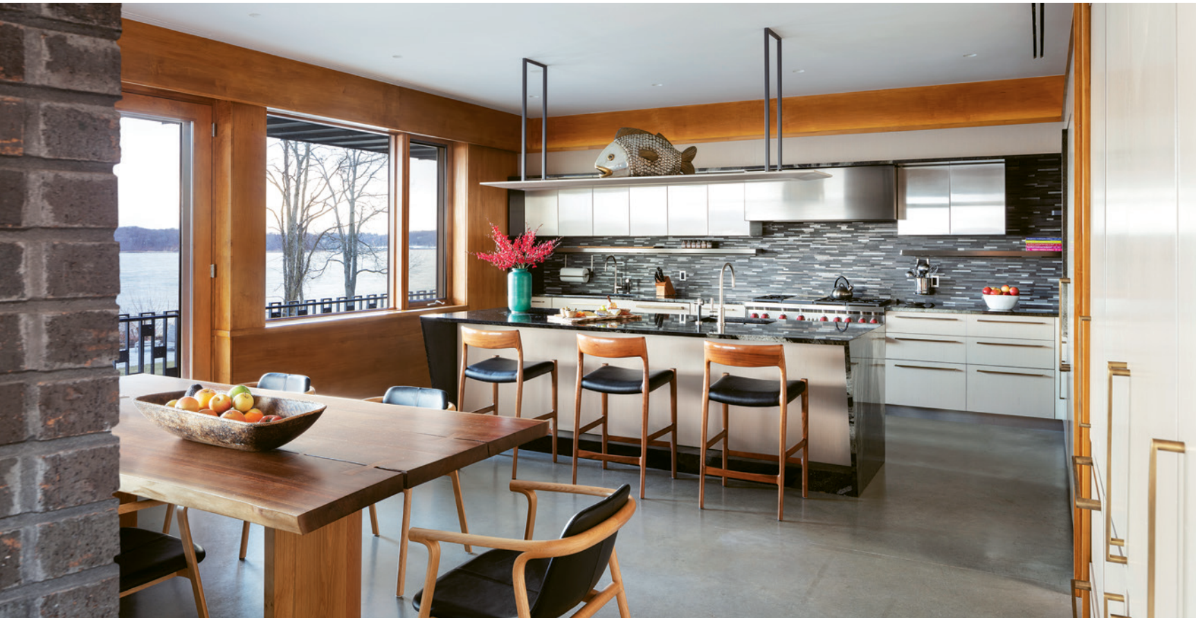
This page: The corner column is part of the steel structure with steel bracket shelves added. An LED strip behind it silhouettes the column at night. Upper cabinets have stainless steel fronts, part of the appliance vocabulary. Base cabinets are a lighter vertical-grain plywood.
