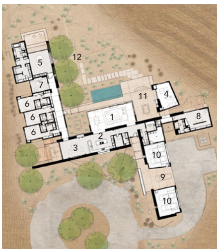
FLOOR PLAN | 1. Great Room | 2. Kitchen 3. Family Room | 4. Game Room | 5. Master Suite 6. Bedroom | 7. Study | 8. Guest Suite/Studio 9. Guest Carport | 10. Garage 11. Covered Patio | 12. Landscaped Court
