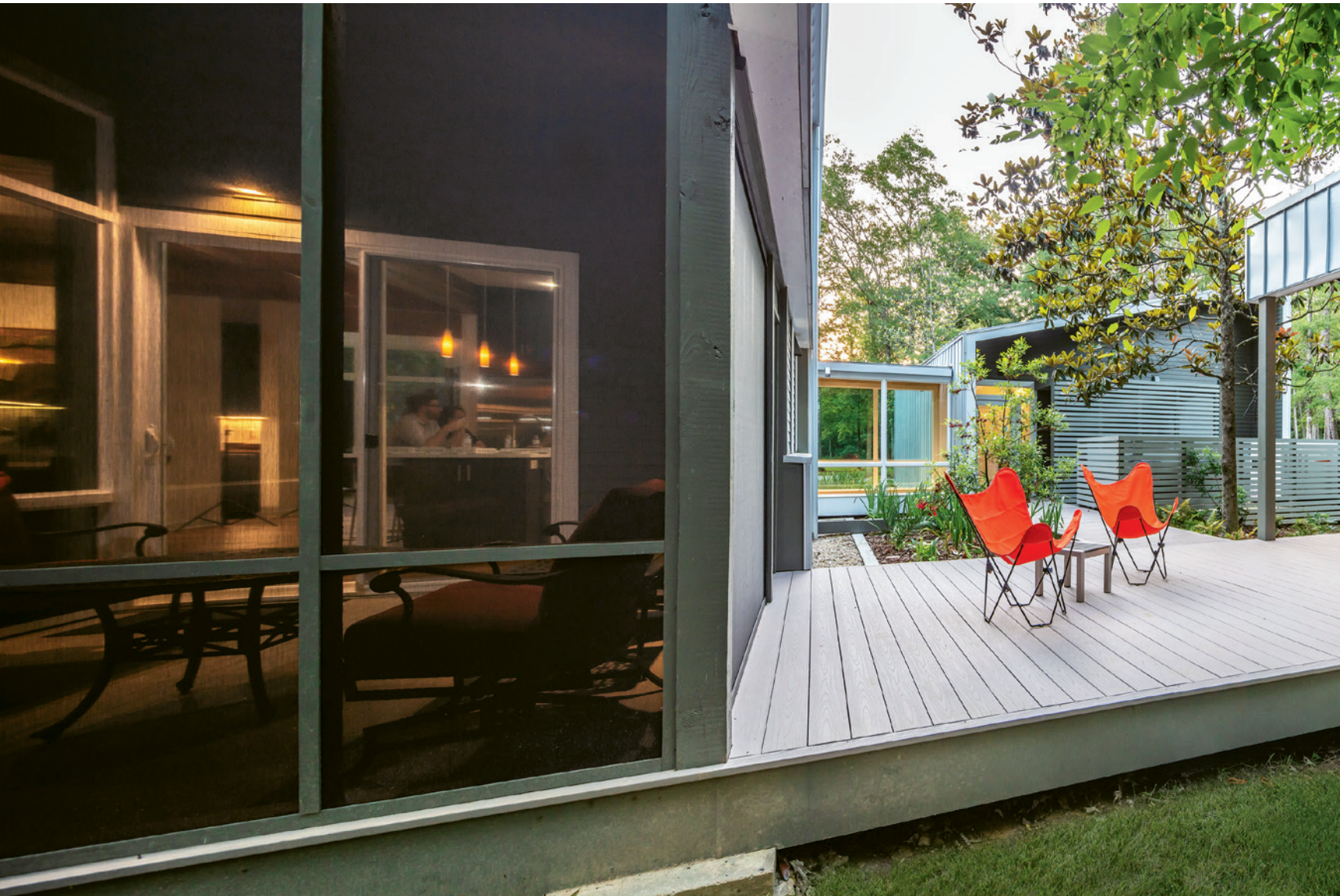
This page and opposite: The house tiptoes across a natural bioswale. Portions of the structure are elevated off the ground to direct water flow toward the nearby creek. A screened porch can open fully to the outdoor kitchen and entertaining area.
