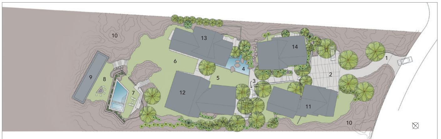
SITE PLAN | 1. Driveway | 2. Auto Court | 3. Outdoor Dining & Kitchen | 4. Koi Pond | 5. Axial Monkeypod Tree | 6. Activity Lawn With Ocean View 7. Pool/Spa | 8. Fire Pit | 9. Bocce Court | 10. Lava Field | 11. Garage/Recreation Room | 12. Living Hale | 13. Master Bedroom Hale | 14. Guest Hale
