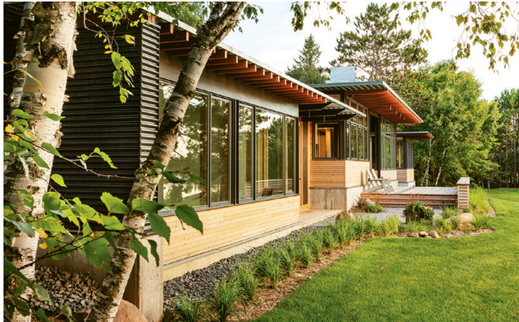
This page: The best views of the lake are westerly, requiring deep overhangs to shade interior spaces from afternoon glare. Hidden steel beams ensure the roof can support seasonal snow loads.
