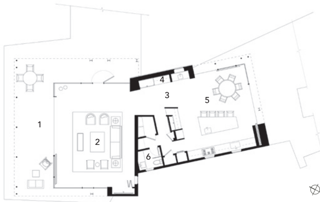
LIVING HALE FLOOR PLAN | 1. Lanai | 2. Living Room | 3. Hall | 4. Wet Bar 5. Kitchen/Dining | 6. Powder Room
