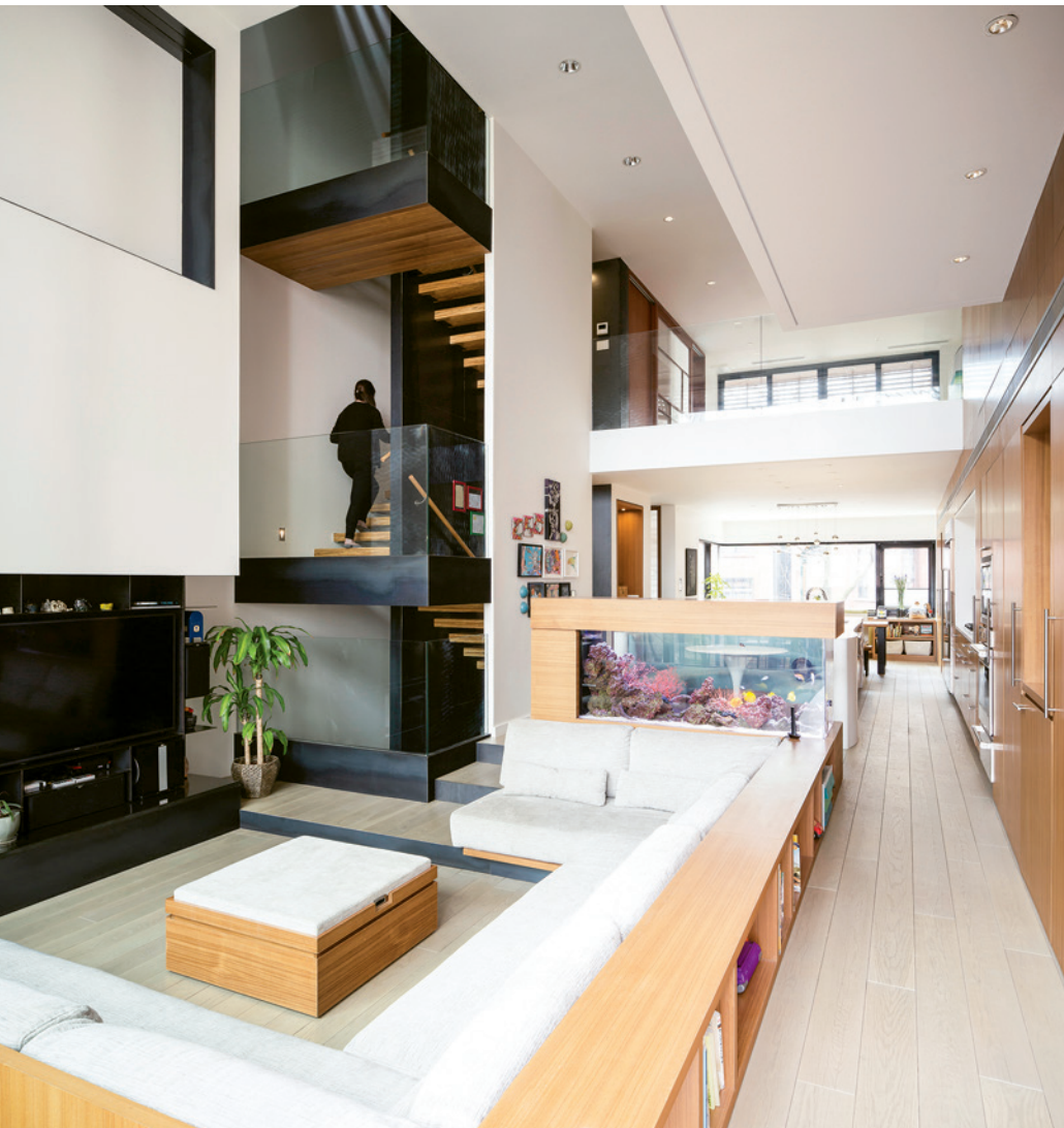
This page and opposite: With its Escher-like maze of sunken levels, mezzanines, terraces, and overlooks, the house draws in abundant natural light. The stairwell's stack effect couples with top-level sliding doors to ventilate the home naturally.
