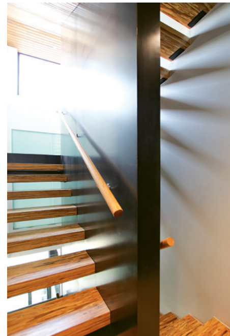
This page and opposite: With its Escher-like maze of sunken levels, mezzanines, terraces, and overlooks, the house draws in abundant natural light. The stairwell's stack effect couples with top-level sliding doors to ventilate the home naturally.
