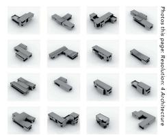
Above and right: The prefab 2017 North Fork Bluff House employs the Z-Type series of modules (module typologies pictured top right), with side wings positioned to block views of the neighbors from the front porch and rear pool deck. The 5,100-square-foot house overlooks Long Island Sound.
