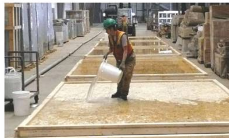
Ainsworth performed a "flood test" on pointSIX, flooding the subfloor for 14 days, simulating extreme, wet jobsite conditions. Yet the OSB experienced swelling equal to not much more than a sheet of paper.
