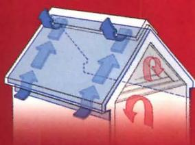
DuPont™ Tyvek® AtticWrap™ helps keep moisture introduced by ventilating air away from the roof structure and ceiling insulation.
