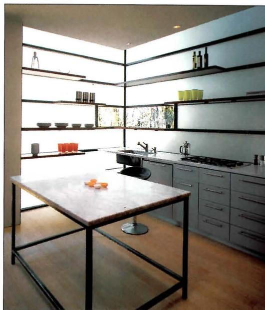
To bring light to this dark row house, David Jameson, AIA, inserted 1¼-inch-thick acid-etched glass into a thin-profile steel volume. Transparent vertical glass panels permit views to the rear and sides of the site.
