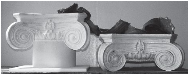
Abatron's MasterMold 12-8 liquid-polyurethane moldmaking compound is used for one- and two-part molds with deep undercuts.
