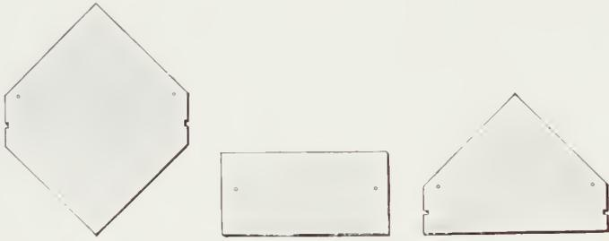
The exact shape of French Method shingle, and the two starters used with it.
