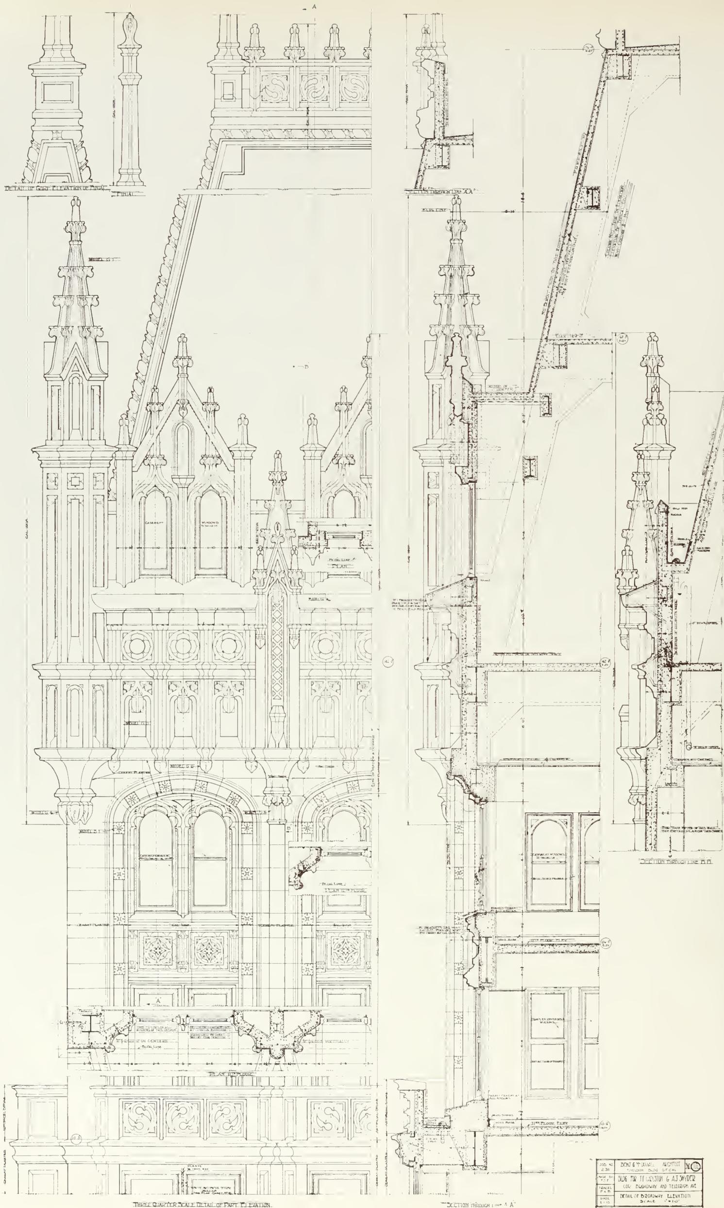
THREE-QUARTER SCALE DETAIL OF PART OF ELEVATION.
