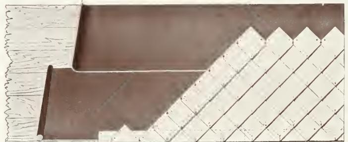
The French Method of using two starters, which is the most common practice.
