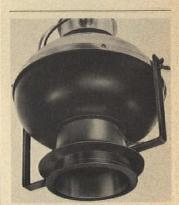
Hidden housing. Recessed, low surface brightness fixtures are designed to produce a fairly high level of illumination from inconspicuous light sources. Specular black anodized cones may be relamped from either above or below and are available in four sizes for lamps between 100w and 300w. Fixture is one of a group of new designs by Swivelier. Swivelier Co., Inc., Nanuet, N.Y. 10954.
