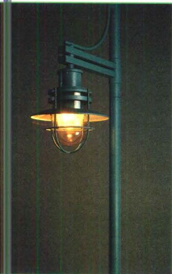
**Outdoor luminaires** from the Mandala Series feature aluminum or steel poles and measure 24 inches in diameter and 17 inches high. The optical systems consist of a round molded polycarbonate or acrylic refractor and a nickel or bronze plated cover. The hardware is corrosion resistant. Lumec.
