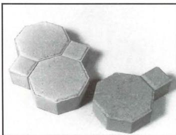
**Concrete paving stones** are now offered in octagonal cobblestones in two thicknesses—2⅜ inch for pedestrian and light vehicular traffic and 3⅜ thickness for heavy vehicular loads. Color options include red, multi-color, brown, buff, and natural. Grinnell.
