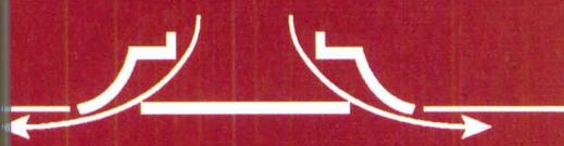
The TITUS® OMNI diffuser projects air in a uniform, horizontal blanket for draft-free heating and cooling, plus protection against ceiling smudging.
