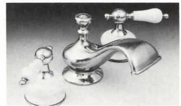
**Decorative faucet series 29** combines a traditional design with a waterfall-like spout. It is available with metal or porcelain handles and escutcheons. The faucets have Epoxy-Glas protection and washerless 1/4-turn ceramic disc brass valves. Harden Industries.
