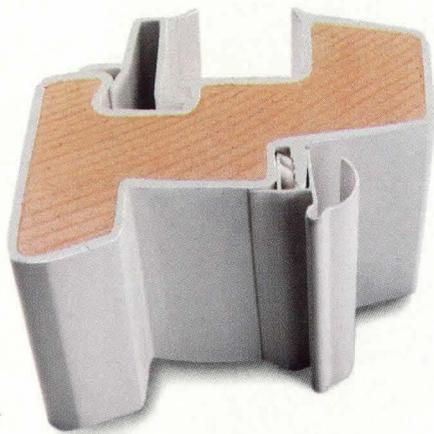
*The Andersen Perma-Shield casement window. Thick, rigid vinyl completely surrounds a treated wood core, protecting it from weathering and wear. The wood core provides superior insulation—the vinyl remains virtually maintenance-free.*
