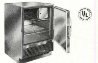
**UC-5** features a two-tray ice cube cooling system with manual defrost and stainless steel defrost water tray. The cooler section has two adjustable stainless steel shelves. The entire UC-5 series features polyurethane insulated thin wall construction and air-tight neoprene thermo-break door seals. Capacity—5.4 cu. ft. (155 ltr.)
