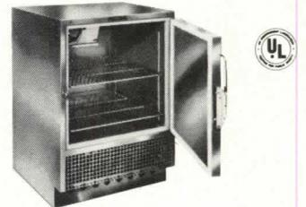
**UC-5-BC** refrigerator has a blower coil cooling system with automatic off-cycle defrosting and condensate evaporator in condensing unit compartment. Two adjustable stainless steel shelves are provided.
