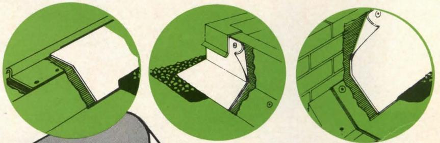
This exclusive *one-ply* Barrett Flashing System was invented to reduce roof problems. The flashing itself is a factory-formed 27-mil laminate of weather-resistant chlorinated polyethylene and strong glass fiber. Specially formulated flashing and lap adhesives complete the system.
