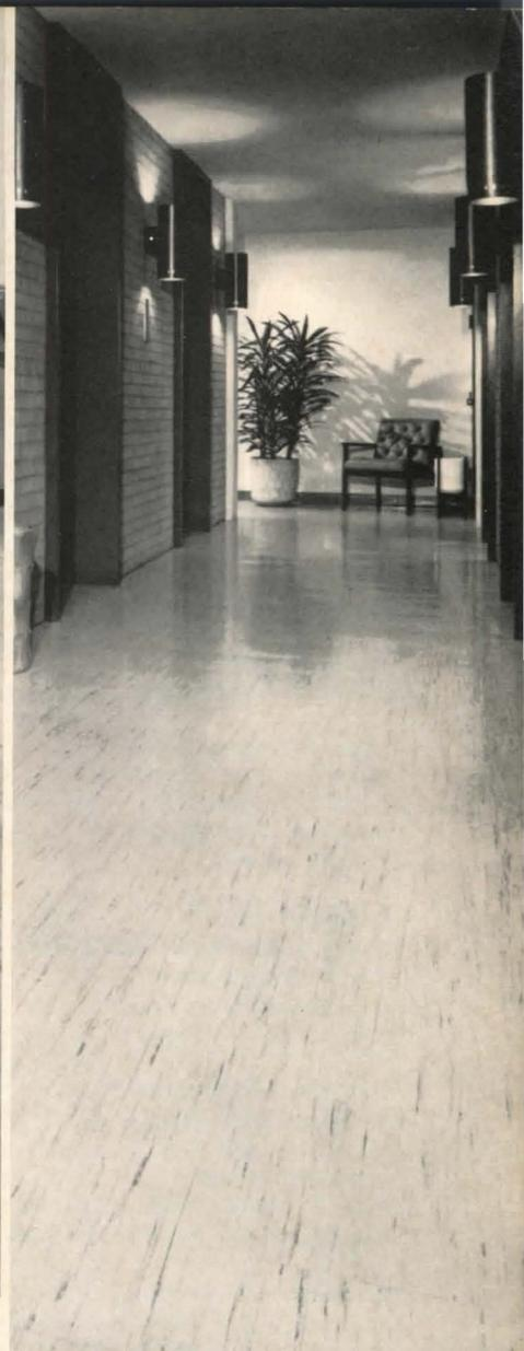
The use of a single Excelon pattern and color throughout the USC installation achieves a pleasing unity of design. And since the graining of the tile runs in one direction, the floor appears seamless. Something else about the graining. It goes all the way through the tile, so it won't fade away or show traffic lanes.
