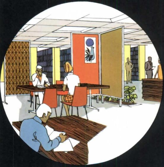
These partitions are called Landscape because they were pioneered by Conwed to implement the concept of office landscaping recently imported from Europe whereby conventional walls are replaced with free flowing, portable partitions to provide ease of communication and arrangement of work areas while furnishing acoustical and visual privacy.
