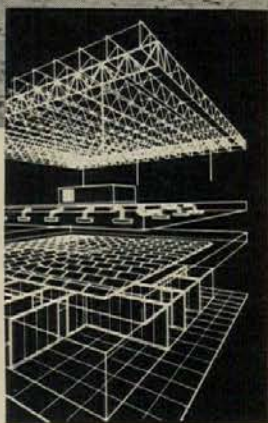
COMPLETE VLMC FRAME for this 47,000-square-foot school—the Robert Frost School in Hyattsville, Maryland—was erected in 11 days. Architect is Ronald S. Senseman of Washington, D.C.
