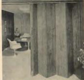
Dual, accordion-fold wood door, "Scale/12 STC (Sound Transmission Class) 25," was developed to stop noise at large openings. Made from 13"-thick, high-density wood core panels with wood or Formica veneer, the door operates on a ceiling track. It is sealed top and bottom with "sweeps" to stop sound. Panelfold Doors, Inc., 1090 E, 17th St., Hialeah, Fla. 33010.
