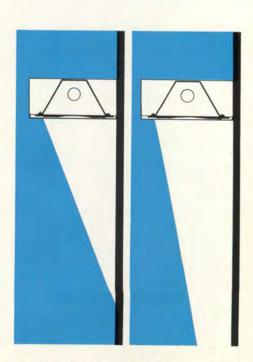
Prismatic structure of the 6044 directs light obliquely at any angle from zero to 15 degrees. allows maximum beam concentration plus even distribution of light on facade.
