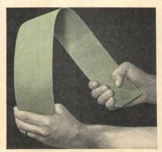
Permanent flexibility. Traffic Topping is resilient . . . expands and contracts without cracking even at temperatures as high as 300°F, as low as -65°F.
