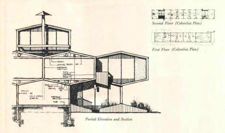
In 1962, William Mileto was asked to design housing for Colombia that could be erected simply, efficiently, and economically. His solution was a system of right-side-up and upside-down trusses and connecting walls that could be slid against each other both backwards and forwards and up and down according to the dictates of varying topography.
