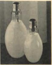
A phosphor coating gives mercury lamps a warm light suitable for indoor use in commercial and institutional applications, claims the manufacturer. The new lamps, called "DeLuxe White," are available in 175-, 400-, and 1000-w sizes. The manufacturer says the color of the light is better than color-improved mercury lamps or cool-white fluorescent lamps. General Electric Co., Nela Park, Cleveland, Ohio 44112
