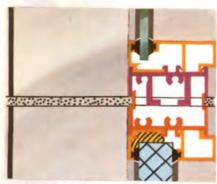
800 System Curtain Wall expands due to extreme summer heat . . . . . contracts due to severe winter cold . . . all expansion and contraction takes place within the module, both horizontally and vertically.
