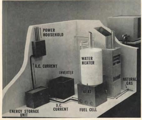
The schematic illustration shows (from right to left): a 5-ton, gas air conditioner; a 100,000-Btuh gas furnace, a 1-kw high-temperature natural gas fuel cell, topped by a water heater that uses the fuel-cell's excess heat, a 10-kw d-c to a-c inverter for supplying the house from the 25-kwh energy storage unit charged by the sure of the feasibility of fuel cells for direct current produced in the fuel cell.
