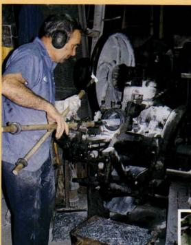
▲ STEP 2: One after another, the steel strips are next attached to long wooden sticks that feed them to the nail-making machines. Each 1870s-vintage machine is geared so it flops the strip back and forth, biting off a nail each time, three to five nails a second.
