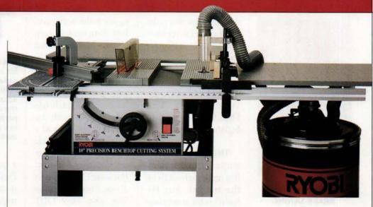
A high-powered "contractor's" saw with a port for mounting a router or jig saw.
