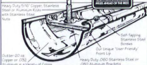
If you appreciate the "Olde World" style of gutters and downspouts and desire to restore and preserve your home in harmony with the original intent of its design. Commercial Gutter systems introduces authentic 6" seamless half-round gutter in both copper & heavy aluminum.
