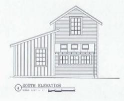
Architect Chris Jenkins's elevations for a garage in Virginia. Jenkins plans on incorporating a combination of plank, lap siding, and smooth Hardy panel with applied battens as well as a terne-metal roof to echo other rural buildings in the area.
