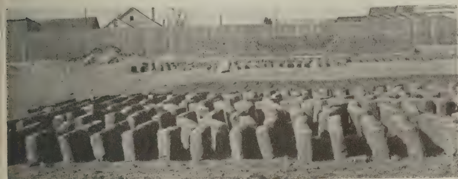
Fig. 6—After a few days the brick are set on edge and allowed to dry further
