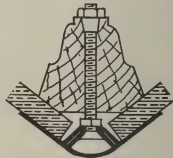
Corner bar showing copper strip outside and wood strip inside on "Desco" store fronts
