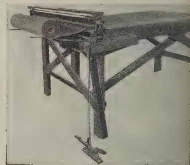
A foot-operated screen wire stretcher
