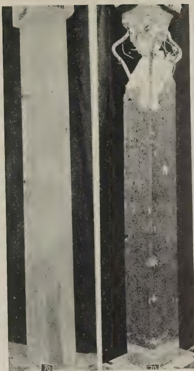
Concrete column before and after test
