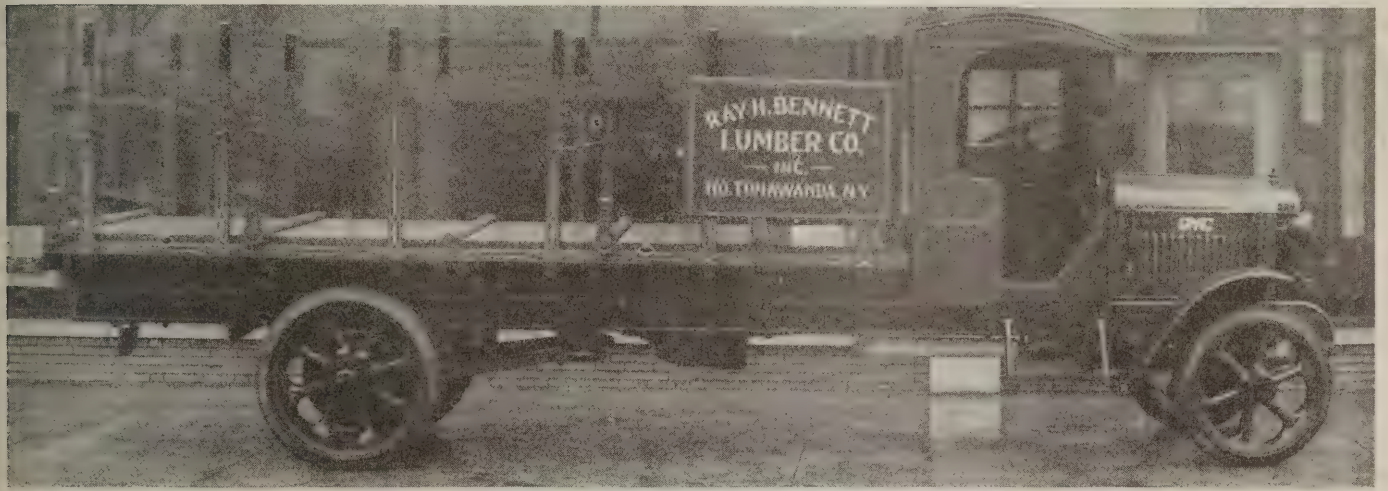
Fig. 4—"Roll-off" body. By means of the rollers an entire load of lumber can be set down at one time
