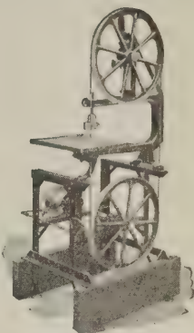
22-inch band saw, tilting table, tension adjustments, upper and lower saw guides. Jewel, $75.
