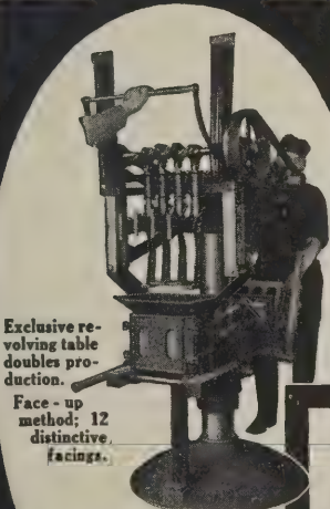
THE NEW UTILITY POWER MACHINE—for Light-Weight Block.
