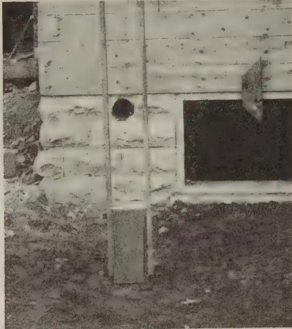
A simple tamper, made from a waste piece of 6x6 and two short pieces of 1x4
