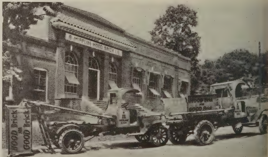
"Fontaine" demountable bodies for handling brick
