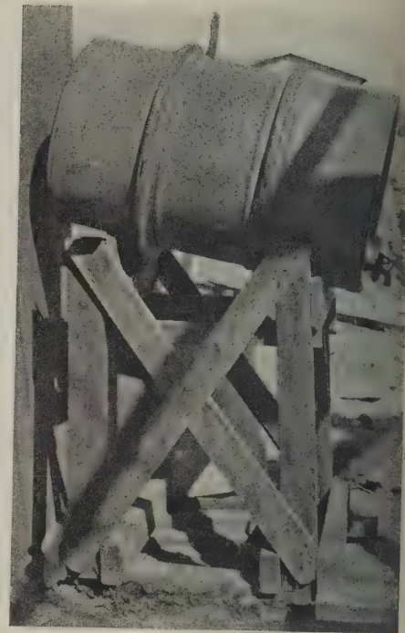
A convenient method for supporting a steel oil drum
