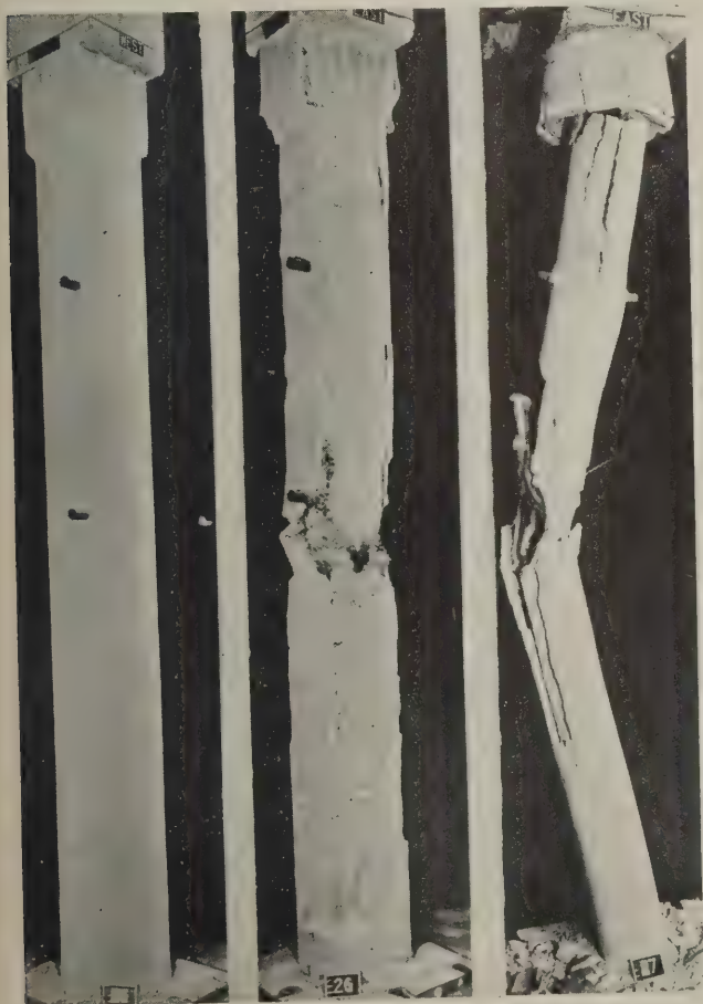
Plaster on metal lath protections before and after fire tests
