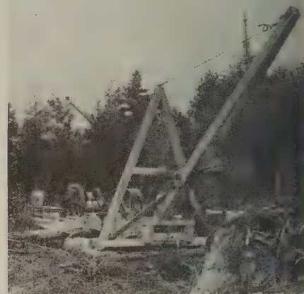
Fig. 3—Combination ditch digger and stump puller
