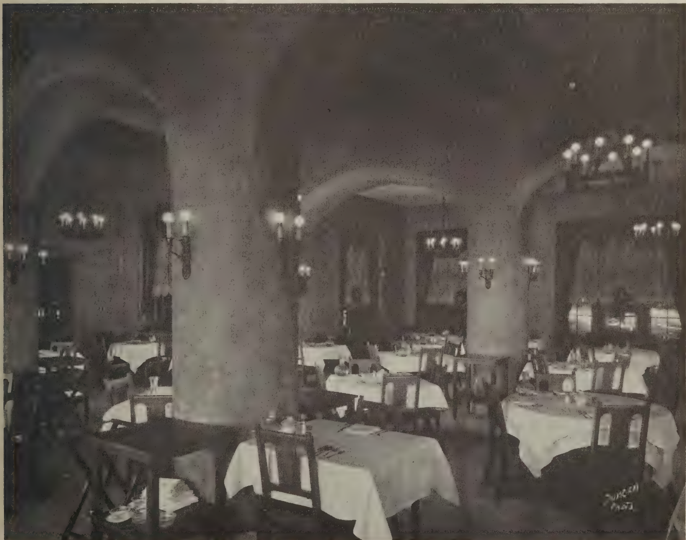
A series of heavy Tudor arches supported by large round columns is used in the dining room. The ceiling is relieved by large wood beams with areas of plaster between. The plaster has a rough finish of parchment shade
