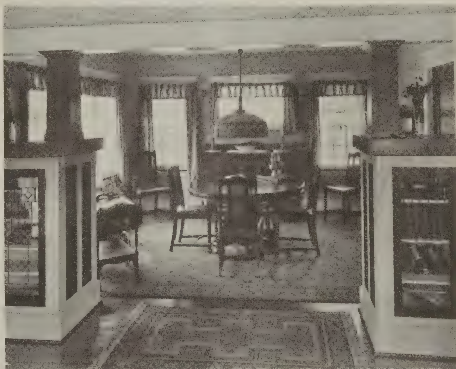
View looking in dining room from living room shows open construction around bookcases and mantels. China cabinets are provided on the dining room side back of bookcases. All trim is flat ivory and dark mahogany. The flooring is red oak hardwood, with black walnut border, laid over the rough flooring
