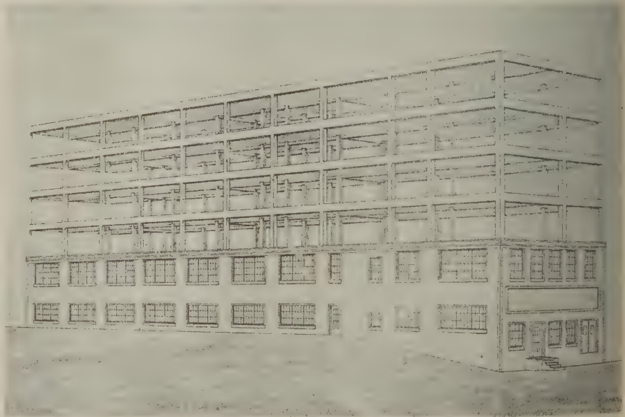
Diagrammatic sketch showing method of construction
