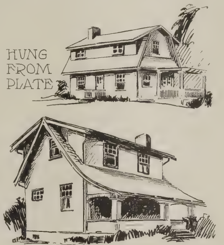
Fig. 6—Overhung roofs and false roofs
