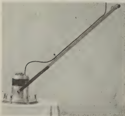
The machine as used for floor work. It is shoved over the work like a plane, releasing on the back stroke
