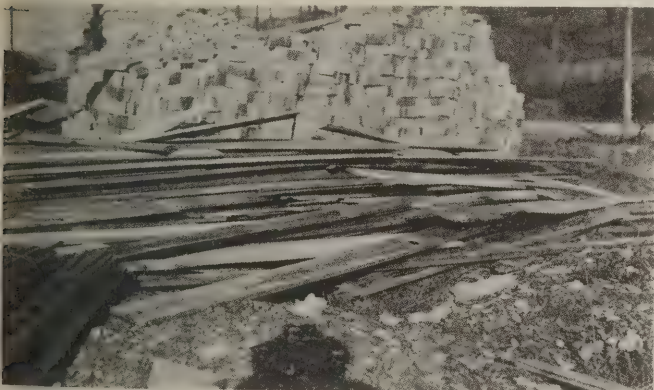
Plate 1—A lumber pile like this invites infection from fungus which may in time cause rot throughout the building
