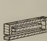
SEC. B MOISTURE DISTRIBUTION SECTION Outer margin sawed off as shown. Outer & center portions weighed, dried, & reweighed separately to determine moisture content.
