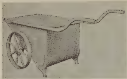
Fig. 7—Concrete charging barrow
